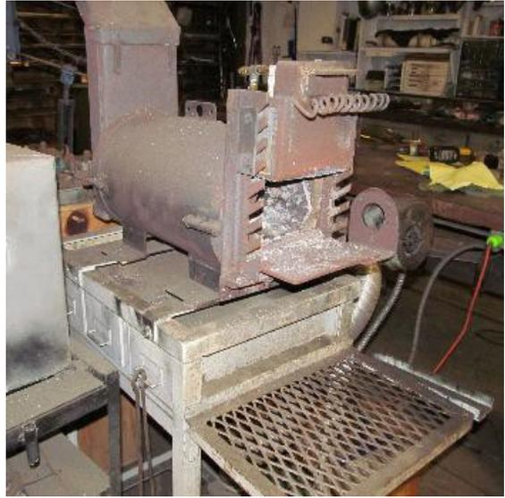
The unit is on a wheeled cart and the lower deck is the site of the blower used for boosting the temperature.
