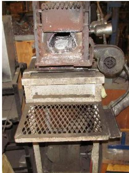
The burners are typical venturi units with 0.040 orifices and can run from 5 to 15 psi of LP pressure. They are inserted in the wall so as to project the flame towards the upper right side of the fire space.
